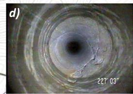
d) Downhole photo from video of "open bedrock" well taken about 150 feet below groundwater. The hole is completely full of groundwater.
